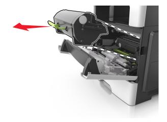
${\bf 3}\,$  Lift the green handle, and then pull the imaging unit out of the printer.
