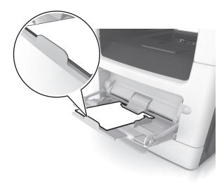
• Load letterhead faceup with the top edge entering the printer first. For two-sided (duplex) printing, load letterhead facedown with the bottom edge entering the printer first.
