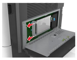
**d** Tighten the two screws.
