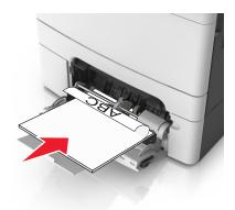
• Load envelopes with the flap side up and against the right side of the paper guide.
