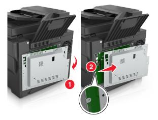
**3** Locate the appropriate connector on the controller board.
